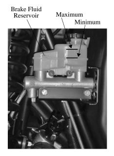
5. Apply the brake forcefully for a few seconds and check for fluid leakage around the fittings.
